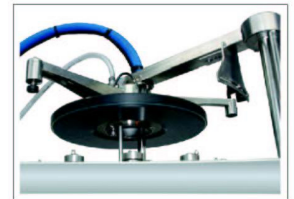
2 Liquid entrance with float and cleaning device
